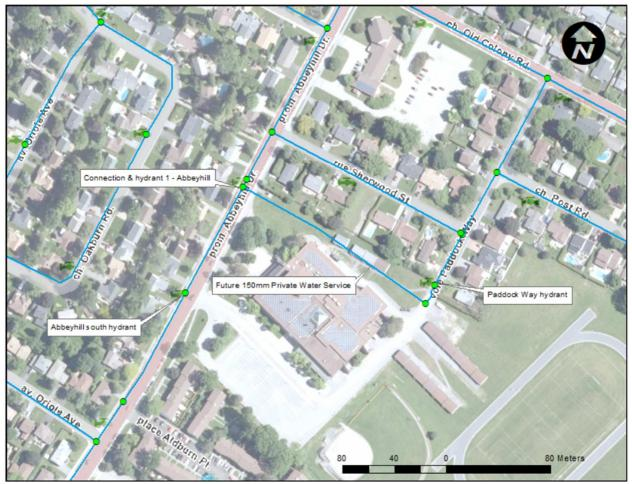
Figure 2: Existing hydrant configuration & connections with future 150mm private water service
