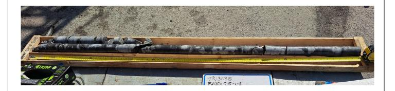
Borehole 25-01 Depth: 13.2 m – 14.6 m Bedrock, Run2, RQD 95%
