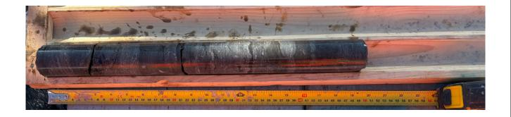
Borehole 25-02 Depth: 11.3 m – 11.8 m Bedrock, Run1, RQD 82%
