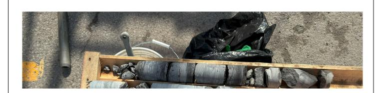
Borehole 25-01 Depth: 12.4 m – 13.2 m Bedrock, Run1, RQD 0%
