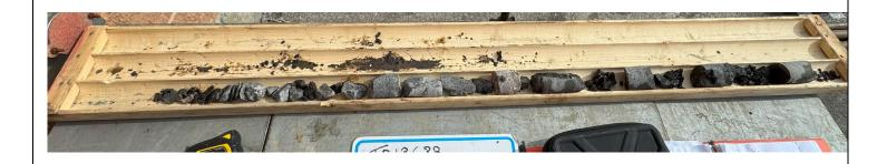
Borehole 25-08 Depth: 17.8 m – 19.4 m Bedrock, Run1, RQD 0%
