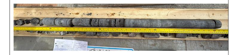
Borehole 25-08 Depth: 19.4 m – 20.6 m Bedrock, Run2, RQD 80%
