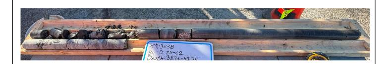
Borehole 25-02 Depth: 11.8 m – 13.3 m Bedrock, Run2, RQD 52%
