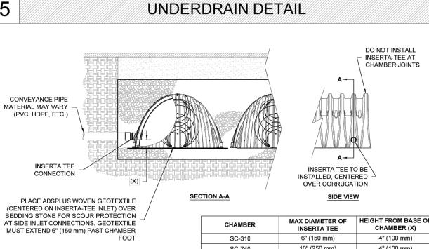
10" (250 mm) 4" (100 mm) 10" (250 mm) 4" (100 mm) 4" (100 mm) DC-780 PART NUMBERS WILL VARY BASED ON INLET PIPE MC-3500 12" (300 mm) 6" (150 mm) MATERIALS. CONTACT STORMTECH FOR MORE 8" (200 mm) 12" (300 mm) MC-4500 12" (300 mm) 8" (200 mm) CONTACT ADS ENGINEERING SERVICES IF INSERTA TEE INLET MUST BE RAISED AS NOT ALL INVERTS ARE INSERTA TEE FITTINGS AVAILABLE FOR SDR 26, SDR 35, SCH 40 IPS
