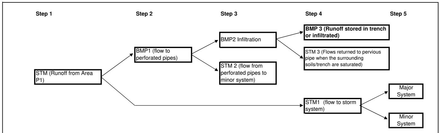
BMP 3 represents the total reduction in runoff volume to the storm sewer system from infiltration through perforated pipes, all other flows are added together and directed to SWM Facility 1.
