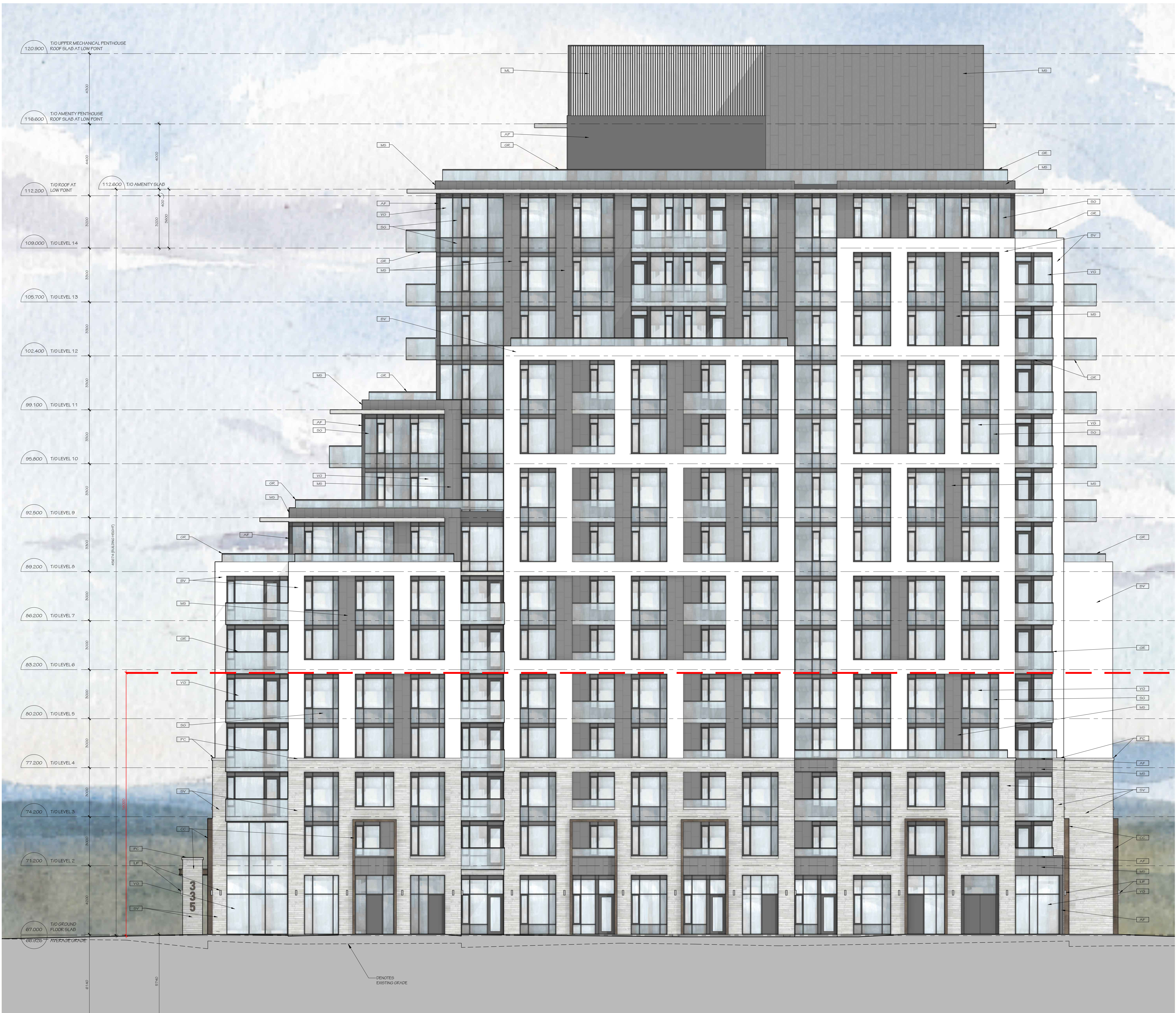
1 WEST BUILDING - SOUTH ELEVATION A3.02 1:100
