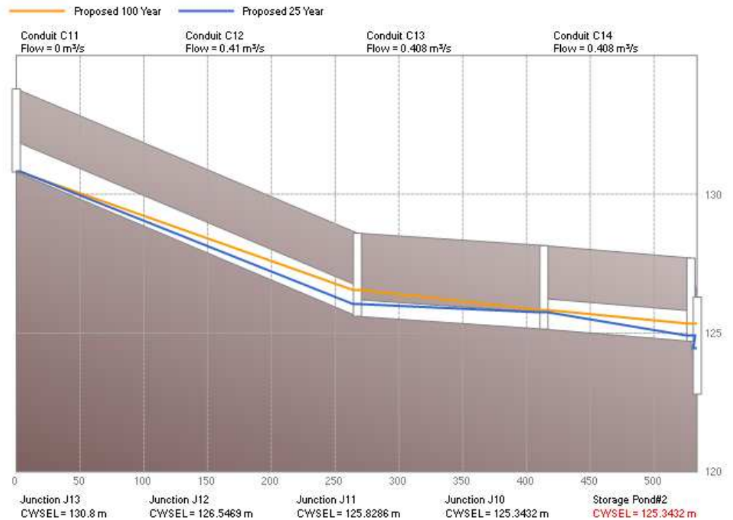
Figure 1: Hydraulic Grade Line along ditch and culvert adjacent to new maintenance building
