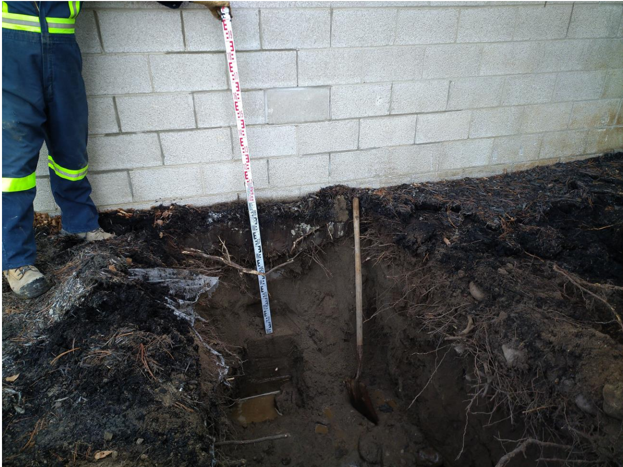
Photograph No. 3: Test Pit No. 1 - Footing Depth
