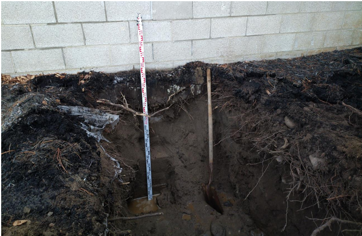
Photograph No. 2: Test Pit No. 1 - Bedrock Depth
