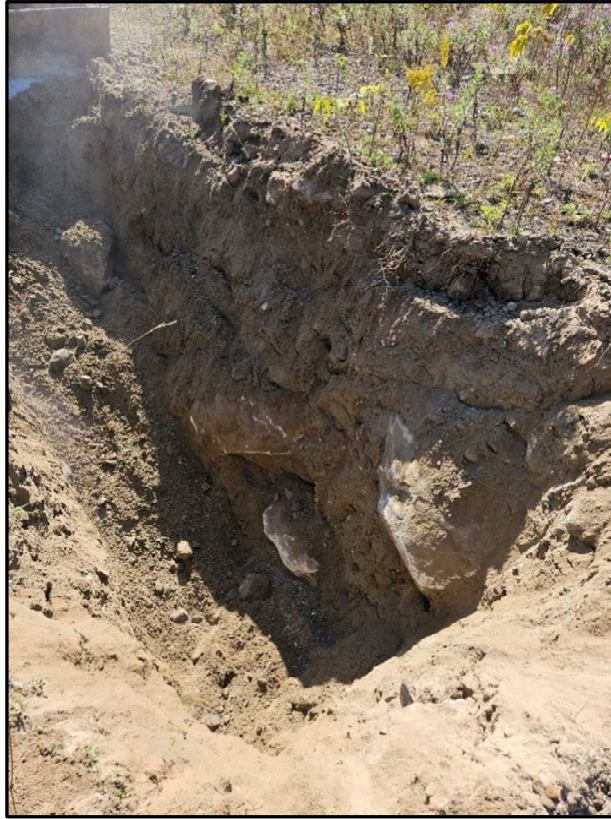
Photo 16: Photo illustrating the boulders excavated from the test pit TP 8-24.
