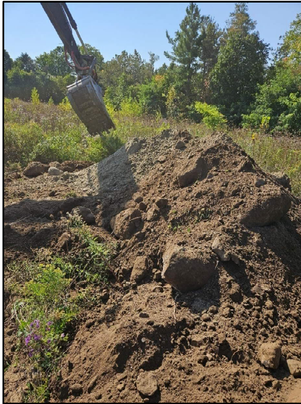
Photo 10: Photo illustrating the boulders excavated from the test pit TP 5-24.
