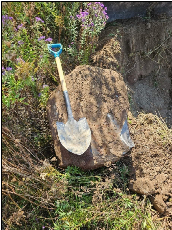
Photo 10: Photo illustrating the boulders excavated from the test pit TP 5-24.
