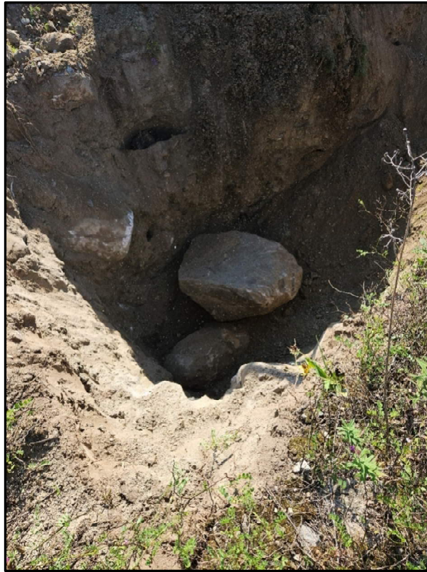
Photo 14: Photo illustrating the boulders excavated from the test pit TP 8-24.
