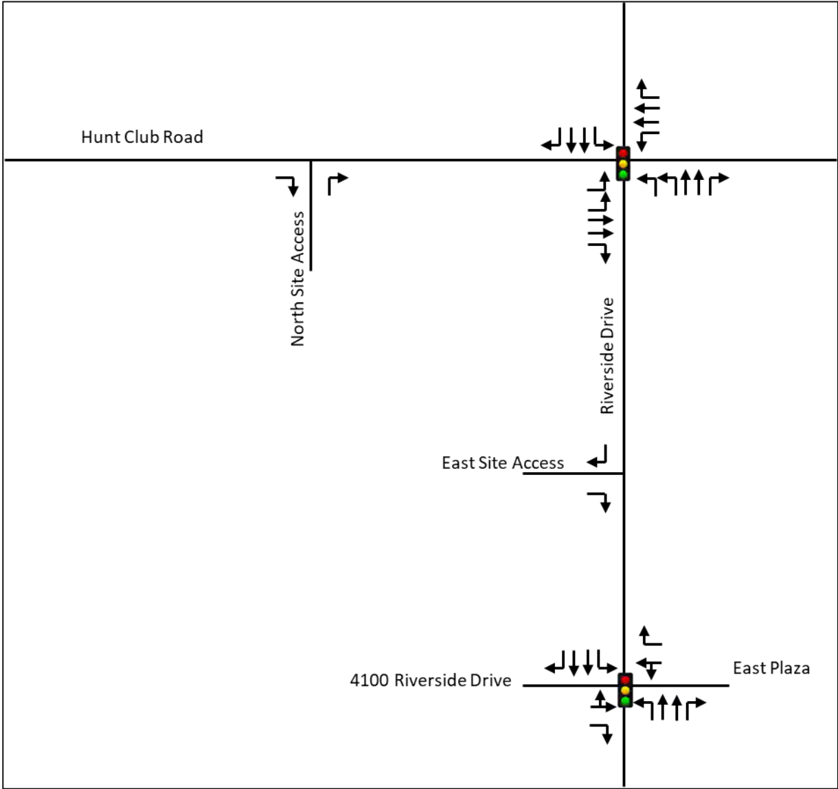
Figure 3 Existing Lane Configuration and Traffic Control
