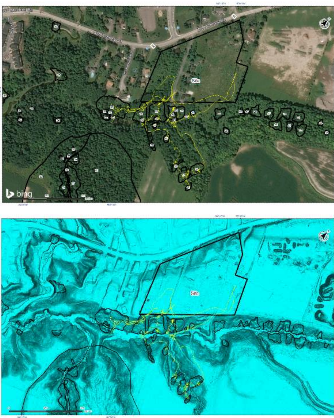
Figure 4-1 Field reconnaissance transect and observed landslide units
