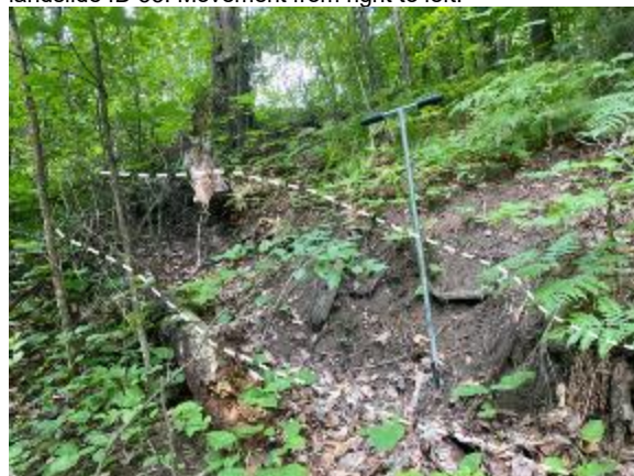
Photo 6: View of a section of the headscarp observed at landslide ID 03, in the area showing movement on the LIDAR change detection.
