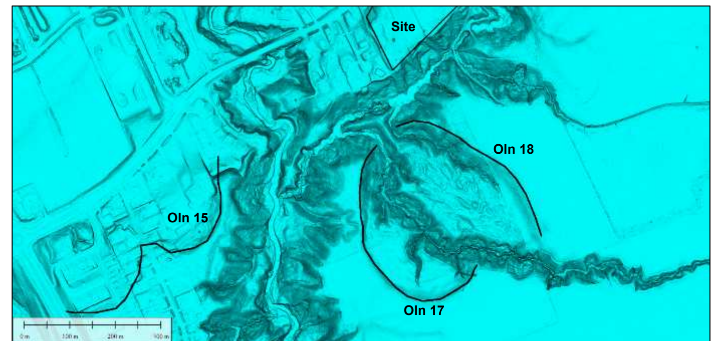
Figure 2-7 2019 bare-earth LiDAR of landslide units OLn 16, 17 and 18
