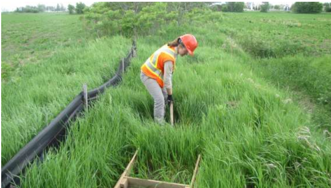
Photo 2: Crew Test Pitting at 5 Metre Intervals, facing south
