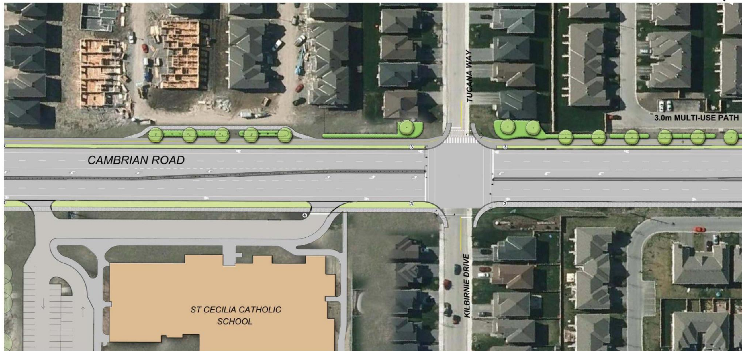
RECOMMENDED PLAN 4-LANE DESIGN ST. CECILIA ELEMENTARY SCHOOL TO TUSCANA WAY/KILBIRNIE DRIVE
