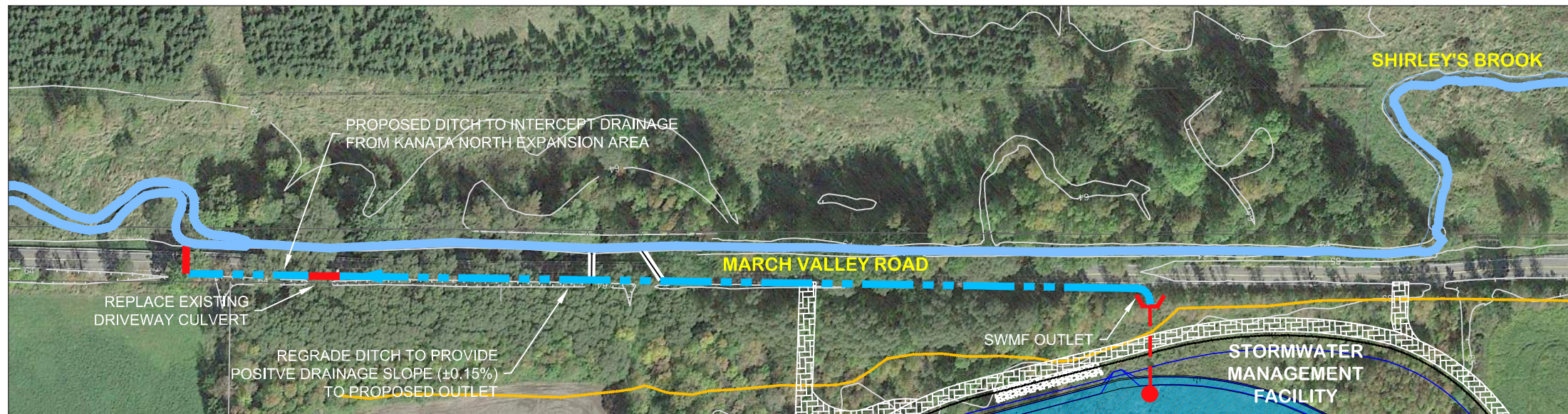
OPTION 1: UPGRADE ROAD-SIDE DITCH SOUTH OF MARCH VALLEY ROAD TO INTERCEPT DRAINAGE FROM PROPOSED SWMF
