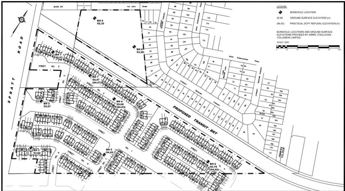
Figure 4: Excerpt from Drawing PG4730-1: Test Hole Location Plan of Paterson Group's Geotechnical Investigation
