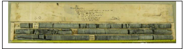
Photo 12 : Borehole BH-04-14, RC-11 to RC-13
