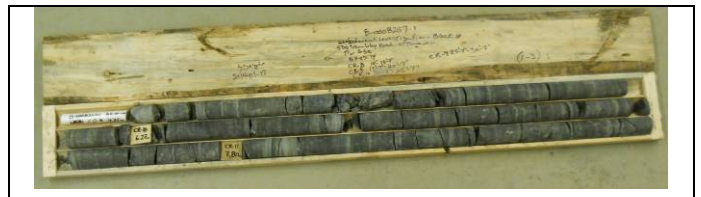
Photo 8 : Borehole BH-03-14, RC-9 to RC-11
