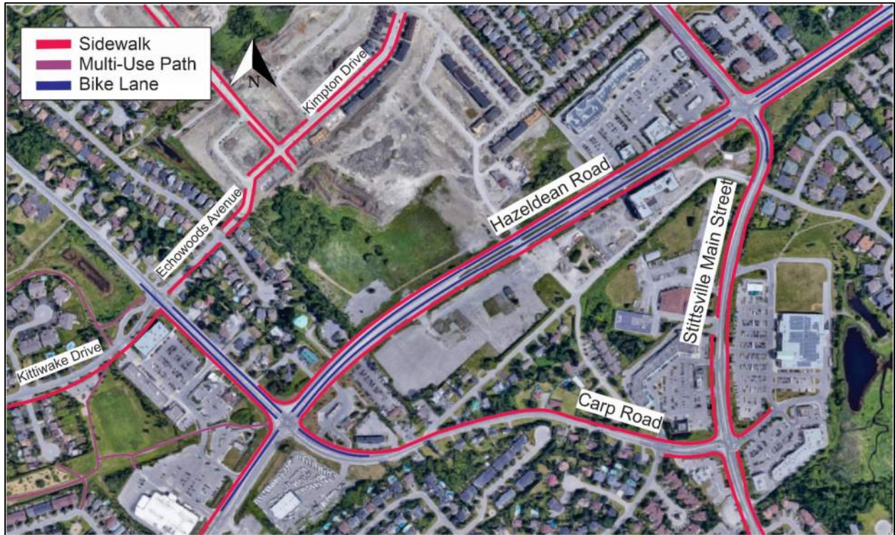
Figure 5 - Pedestrian and Cycling Infrastructure
