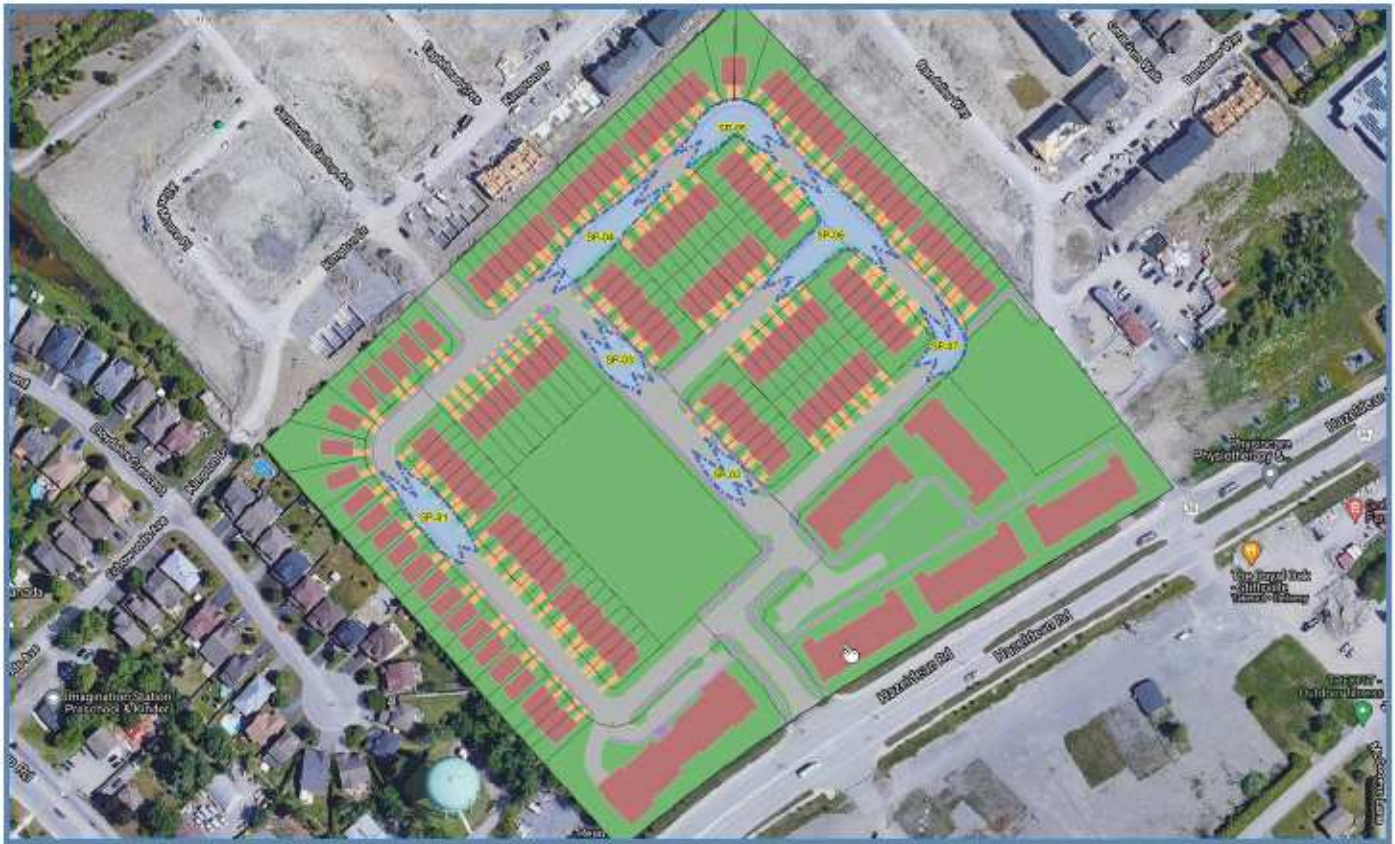
Figure 7-1: Surface Ponding Locations
