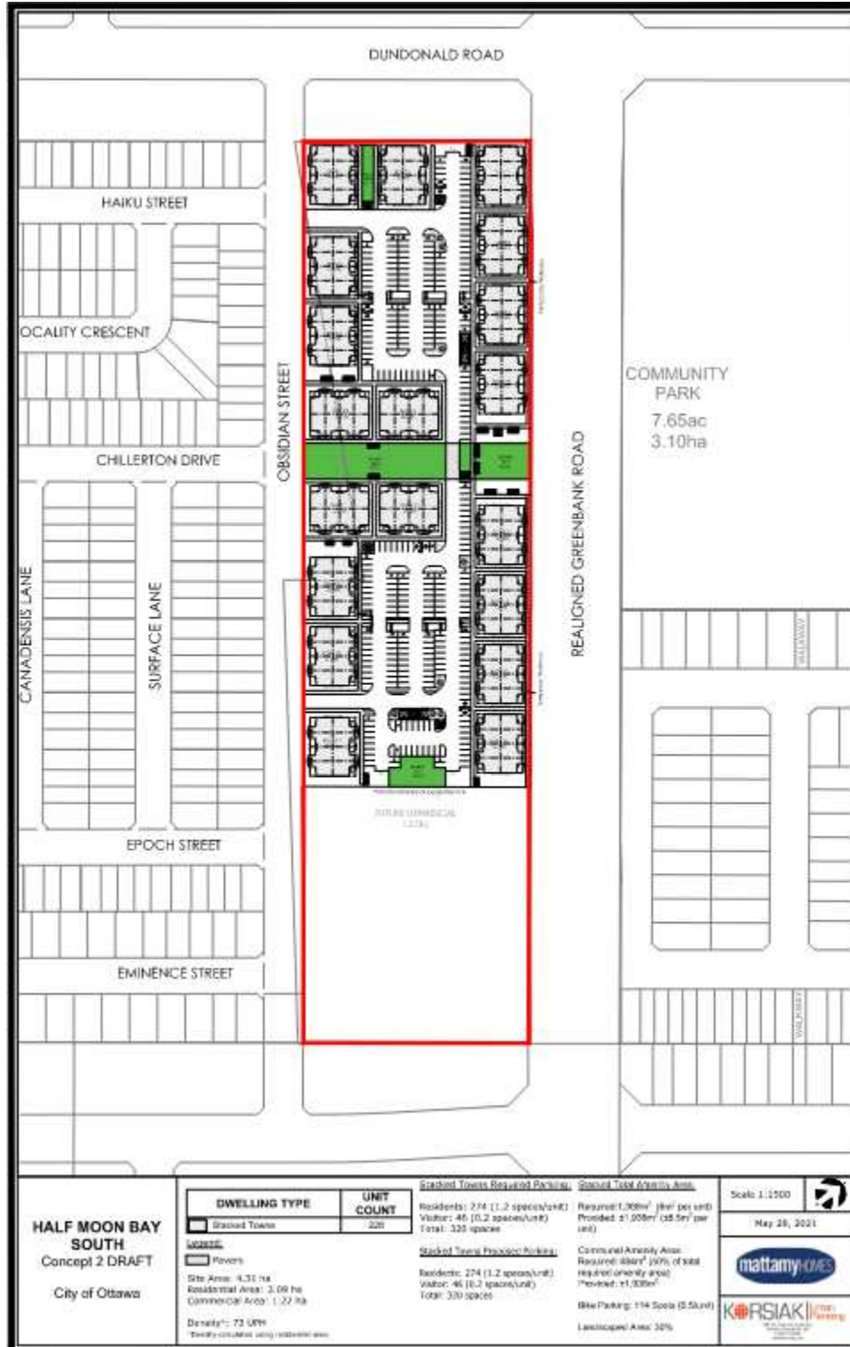
Figure 5: Concept Plan of Block 1 of the proposed development, prepared by Korsiak, dated May 28, 2021
