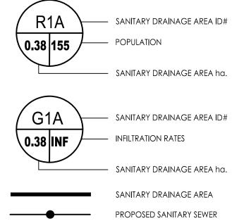
SANITARY DRAINAGE AREA ID# - SANITARY DRAINAGE AREA ha. SANITARY DRAINAGE AREA
