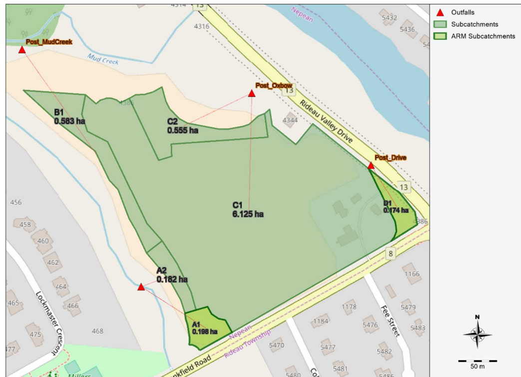
Figure 2: PCSWMM Model Schematic - Proposed Conditions
