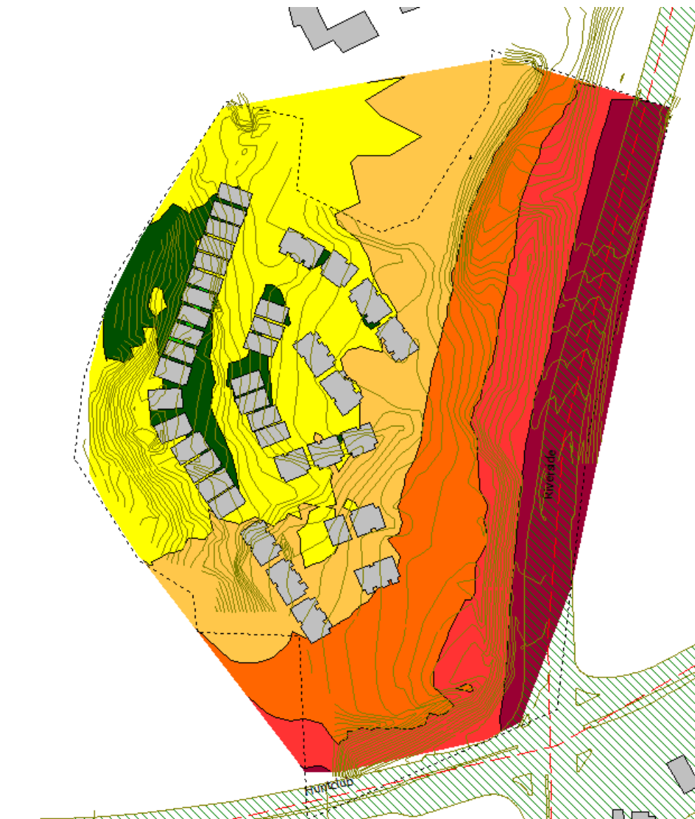
FIGURE 4: NIGHTTIME TRAFFIC NOISE CONTOURS, LOW-RISE ONLY (4.5 M ABOVE GRADE)
