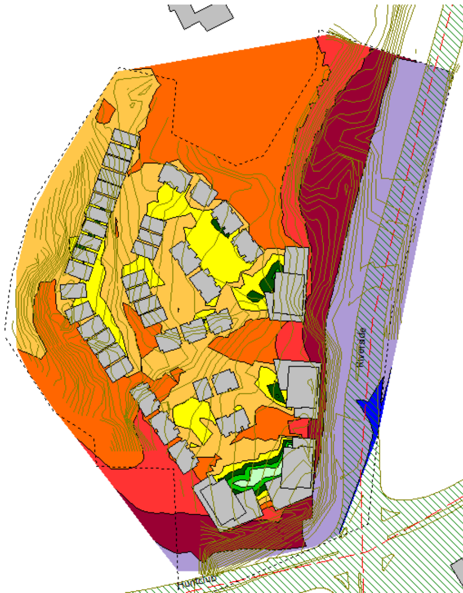
FIGURE 7: DAYTIME TRAFFIC NOISE CONTOURS, WITH MID-RISE (4.5 M ABOVE GRADE)
