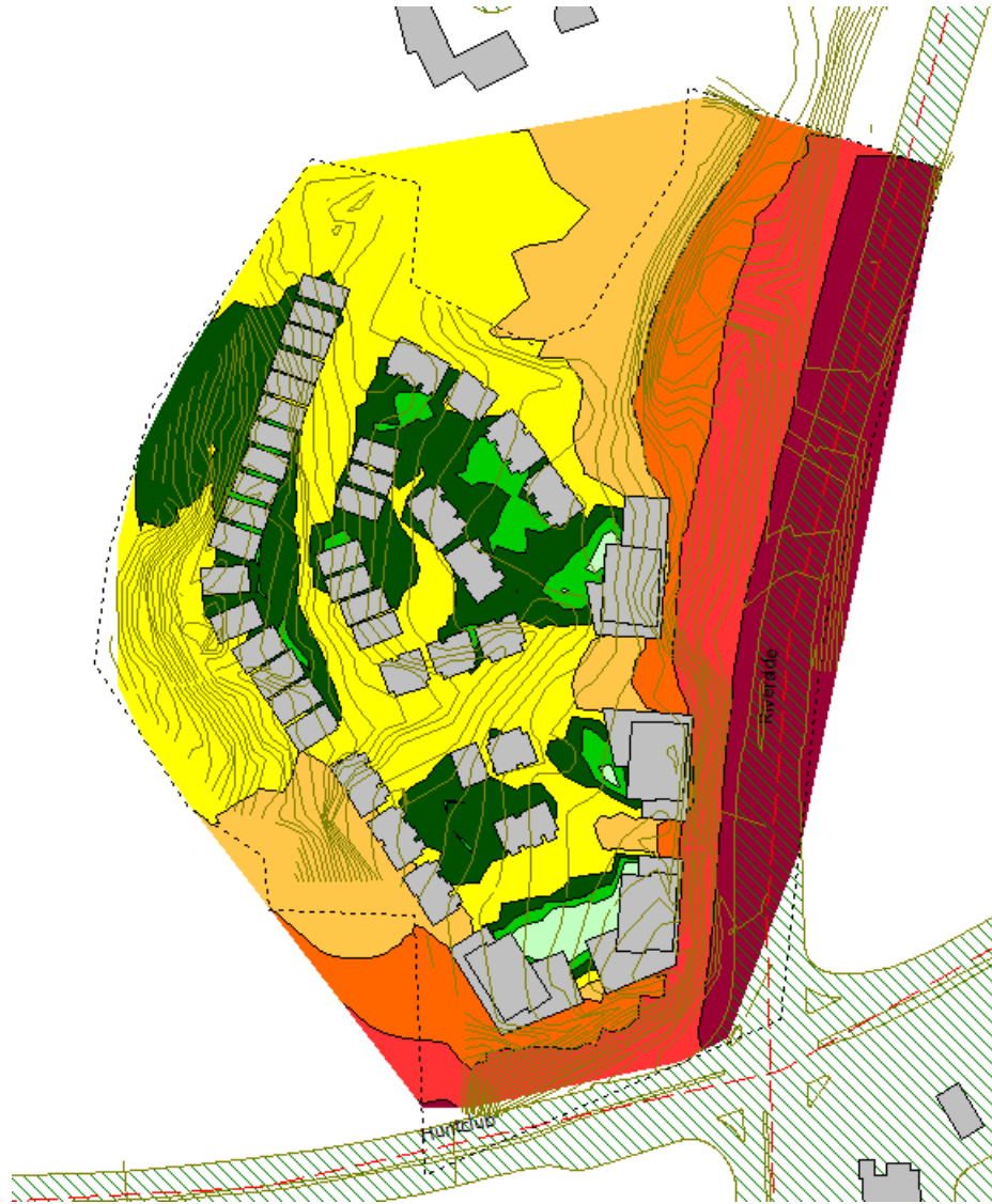
FIGURE 8: NIGHTTIME TRAFFIC NOISE CONTOURS, WITH MID-RISE (4.5 M ABOVE GRADE)
