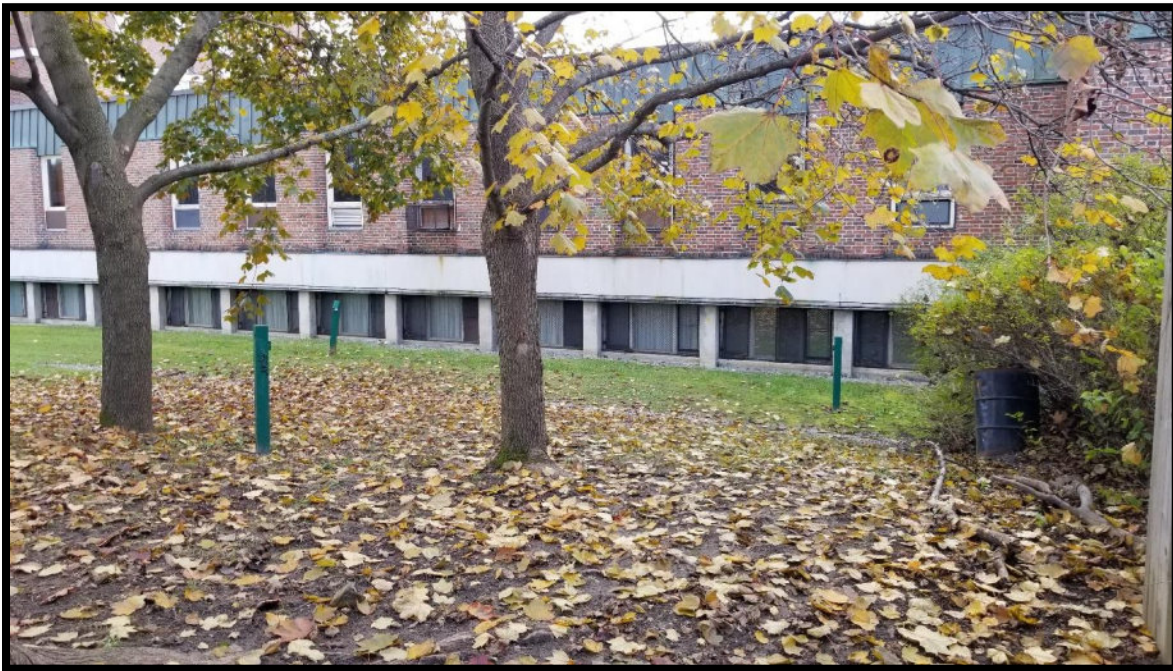
Photograph 5: View of a northern side of Building B. Three (3) monitoring wells, installed by DST in 2015, can be seen (facing south).
