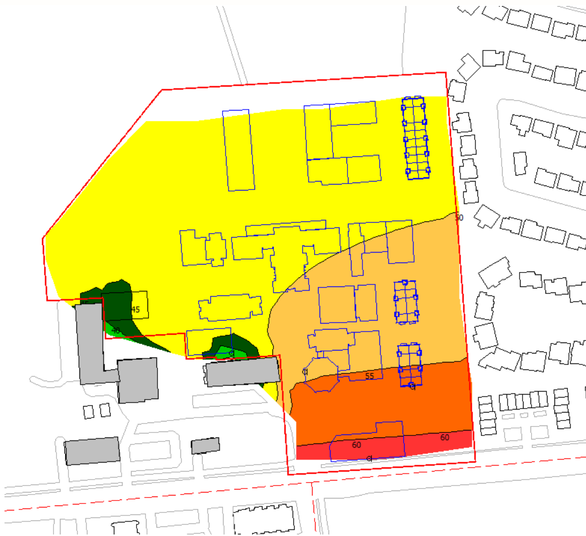
FIGURE 7: NIGHTTIME NOISE CONTOURS (4.5 M ABOVE GRADE)
