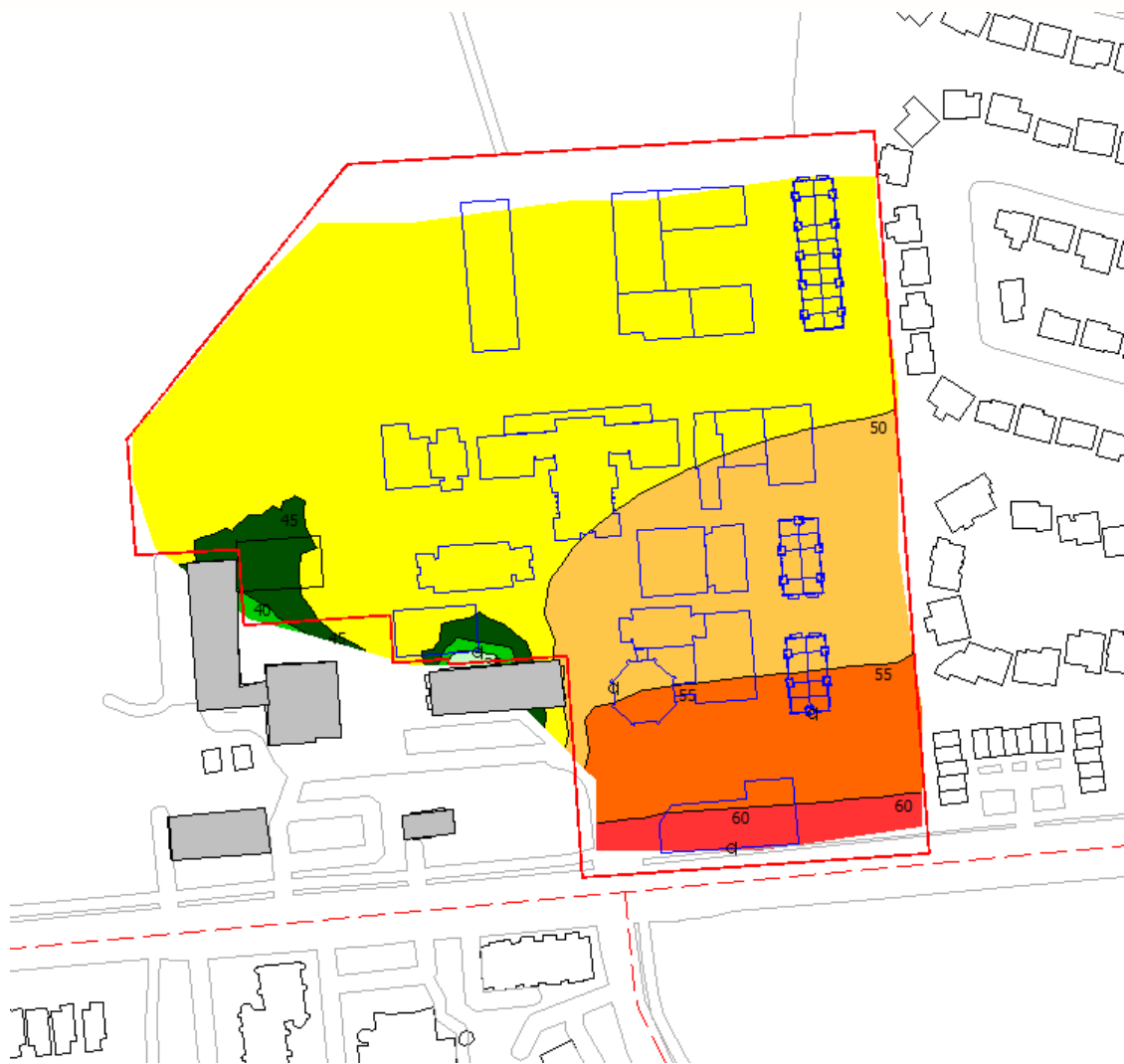
FIGURE 5: NIGHTTIME NOISE CONTOURS (1.5 M ABOVE GRADE)
