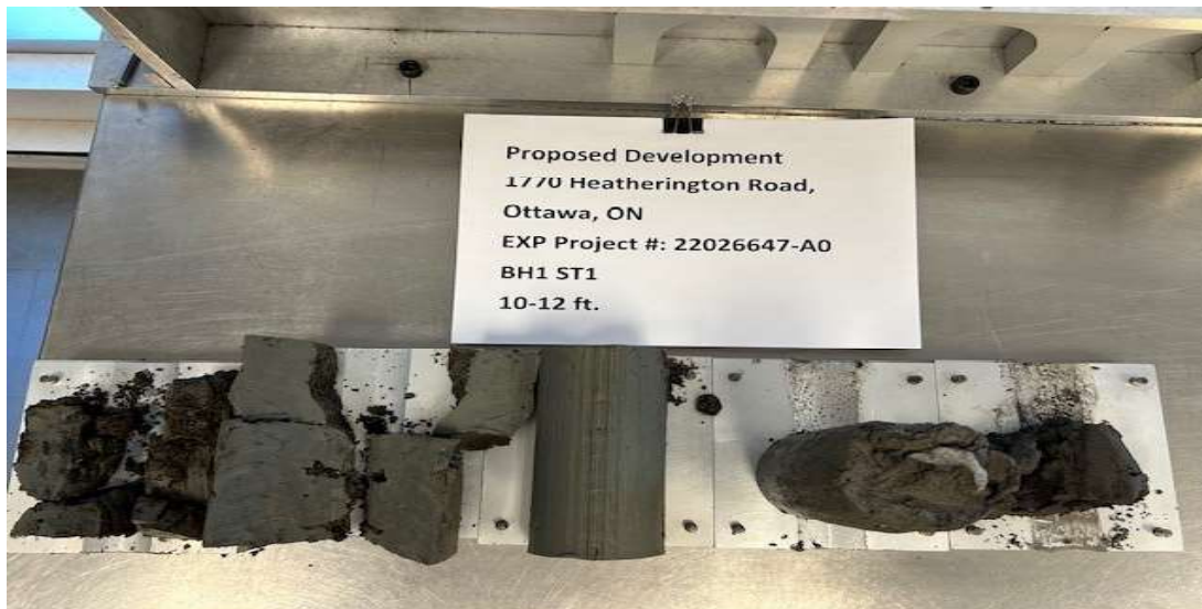
BH1 SS1-Top half of upper section is disturbed; lower half of bottom section is silty clay till
