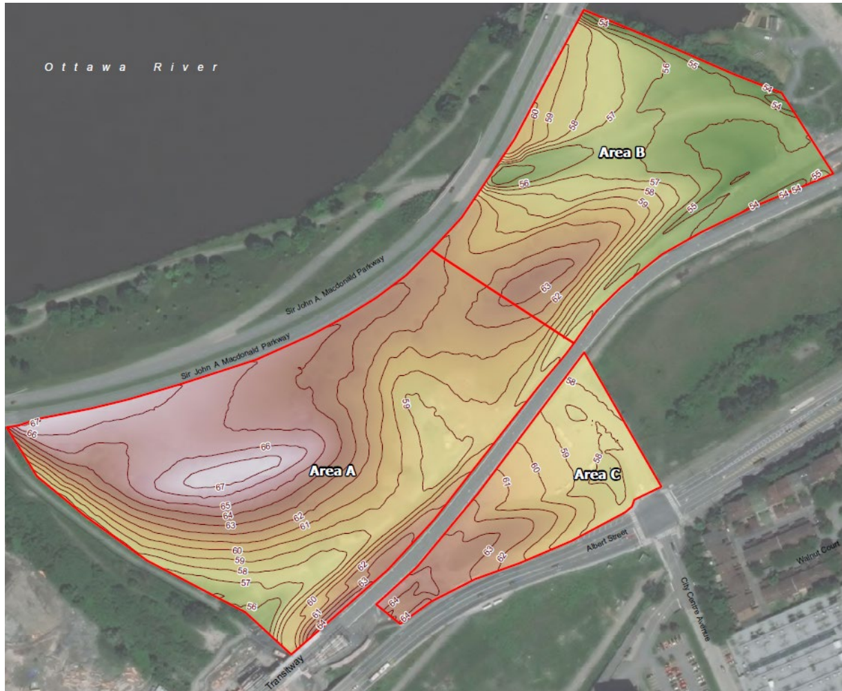
Figure 3.2: Ground surface elevation contours for a portion of the site to the west of the Nepean Bay (Geofirma 2019 report)
