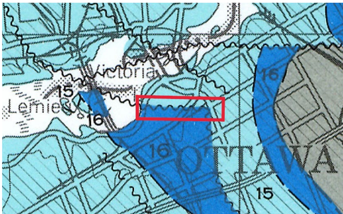
Figure 3.1: The splays of the regional Gloucester Fault at the site area (Bélanger and Harrison, 1976)
