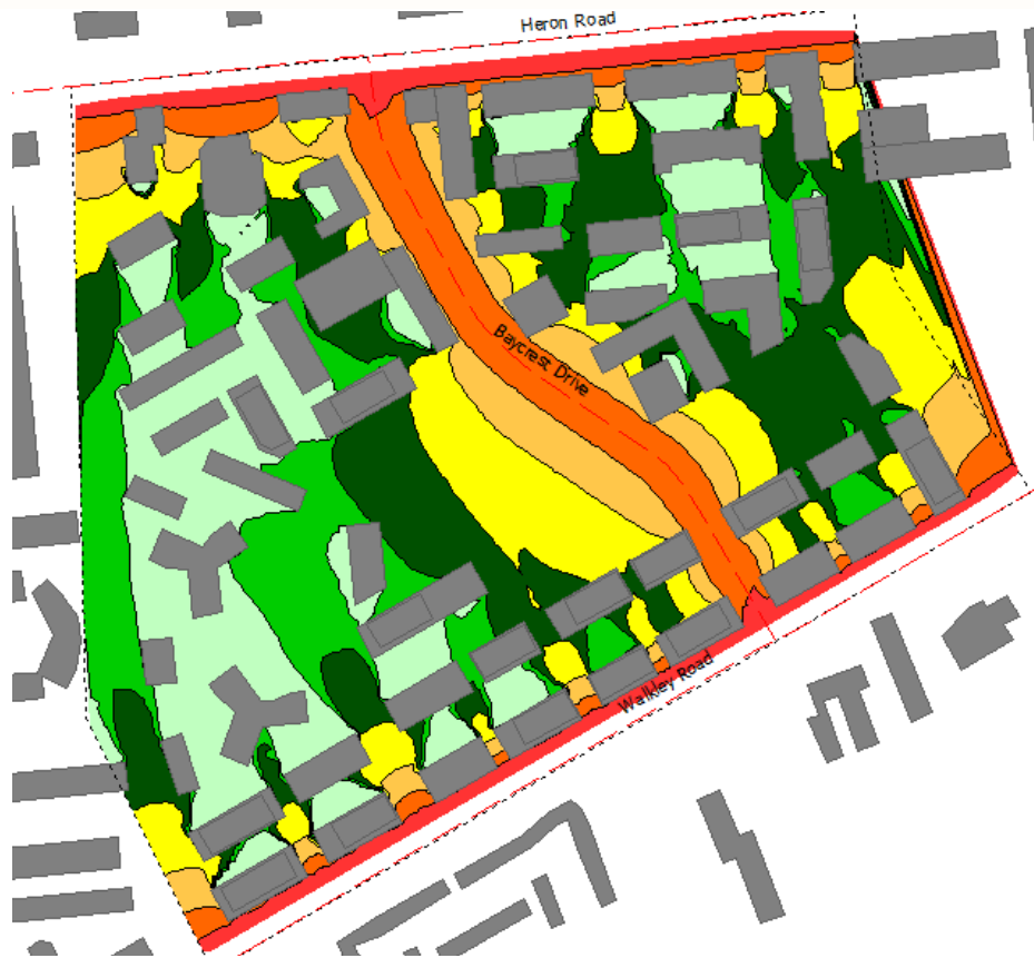
FIGURE 8: NIGHTTIME TRAFFIC NOISE CONTOURS (4.5 M ABOVE GRADE)
