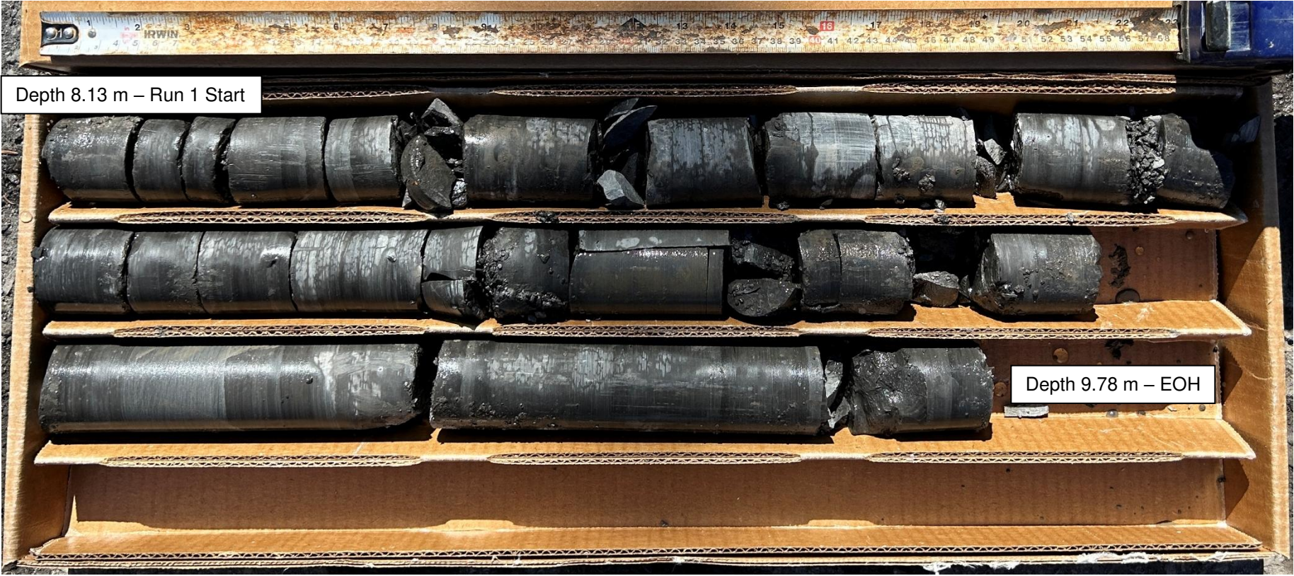
BH105-25 Cored length of 8.13 to 9.78 mbgs Core Box 1 of 1
