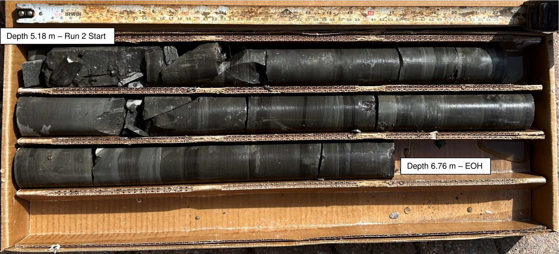
BH101-25 Cored length of 3.43 to 6.76 mbgs Core Box 2 of 2
