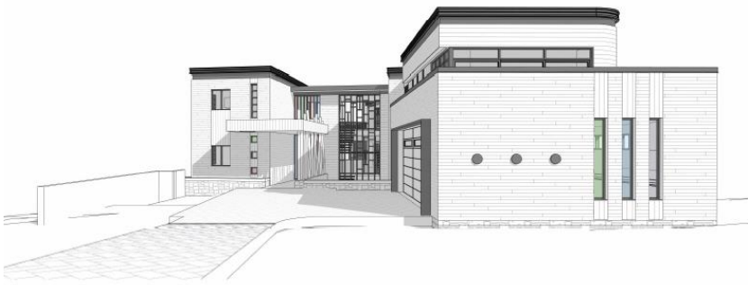
Figures 21: A view of the west elevation from Cloverdale. The garage of the Grade 1 home projects into the notch and creates a pinch point that is compensated for with a side yard setback and shifting of the garage to the opposite side of the lot. The distance of the garage from the grade 1 garage at 384 Cloverdale is 16.8m. Source Linebox Studio.
