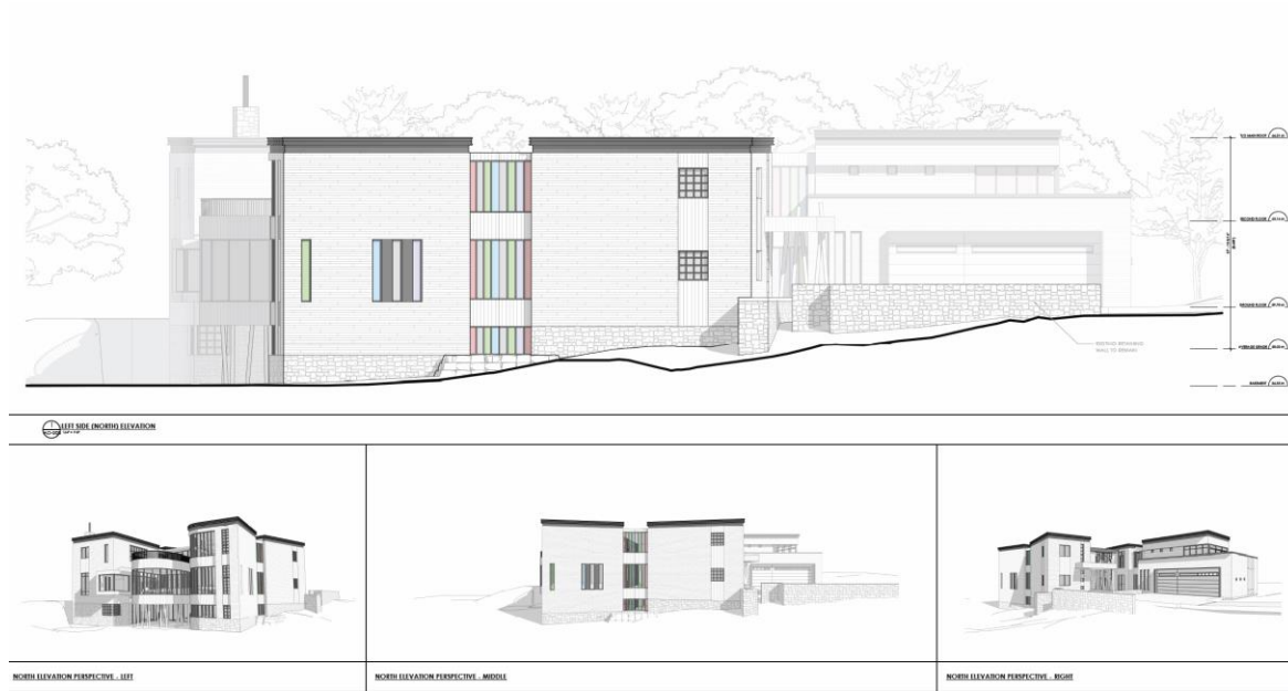
Figure 12: North Elevation from the neighbouring property. On the north side of the property, the proposed home is set back over 23 meters from the street property line to the extent that its’ front edge is in the rear yard of the adjacent property. Existing mature trees and additional trees and shrubbery will buffer the massing from the neighbour. Source Linebox Studio 2023.
