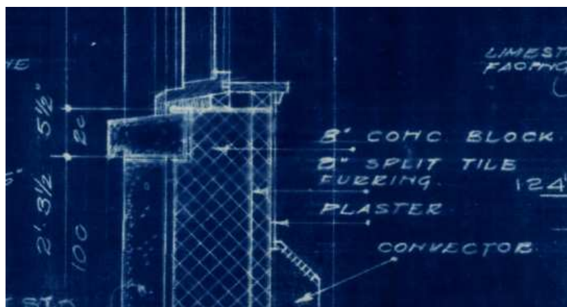
Figure 18; Detail section through the Kent and Gilmour facades illustrating the arrangement of the limestone sill course and limestone cladding. The sills are bonded to the limestone cladding and the concrete back-up wall making it difficult to salvage the windowsill course material. The drip edge only adds to the difficulty of successfully salvaging the material for reuse. Source: 1955 Drawing Set A4
