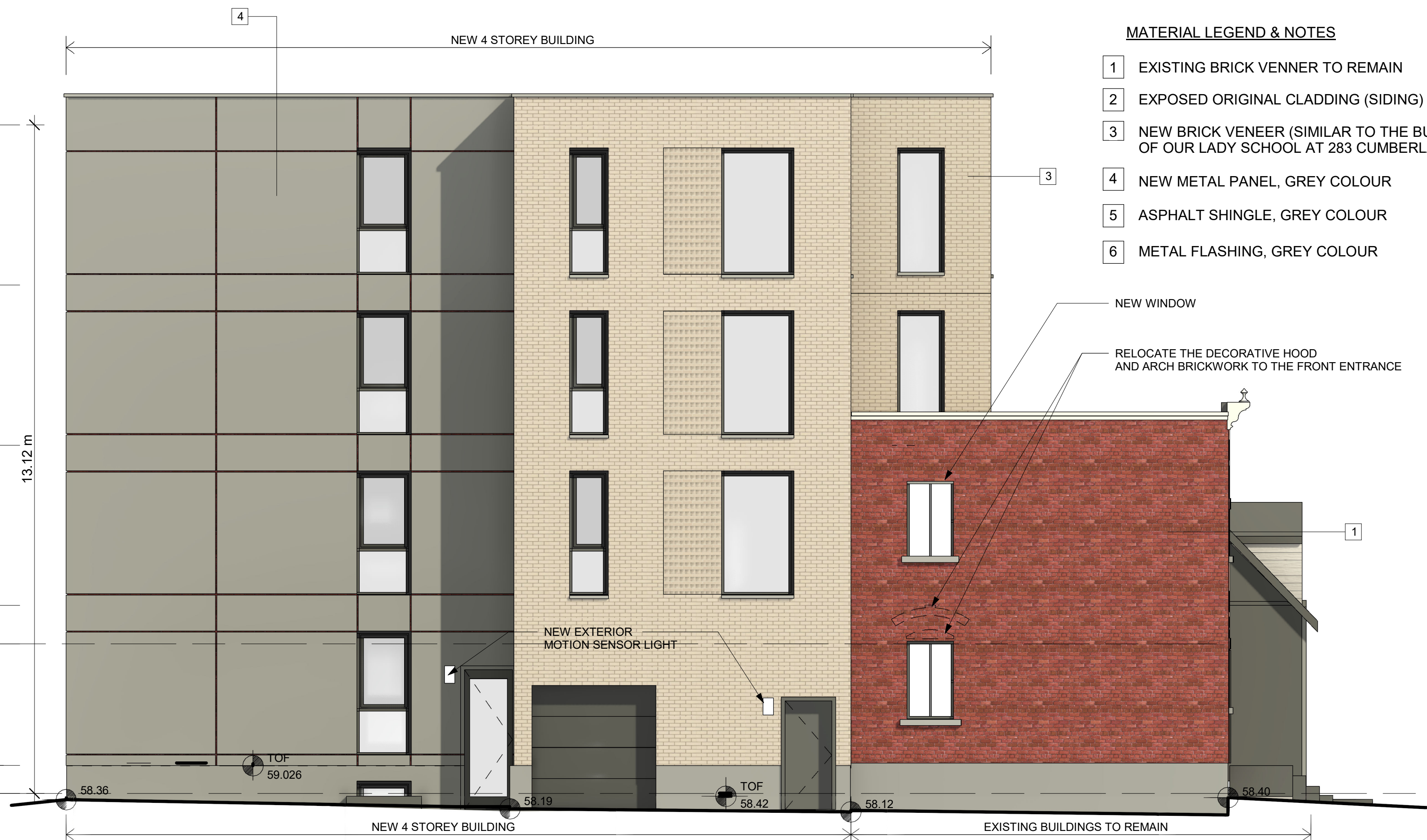
4 Side (East) Elevation 3/16" = 1'-0"
